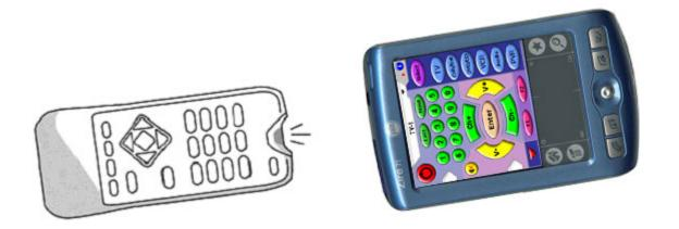
To learn any button, e.g. PiP Ch+, first tap its virtual image on the screen of the handheld. Then press the button "PiP Ch+" on your original remote and hold it until the handheld produces a beeping sound, and then release 'PiP Ch+' button on the original remote. You will notice a change in the button's image on the handheld as you complete this process.
