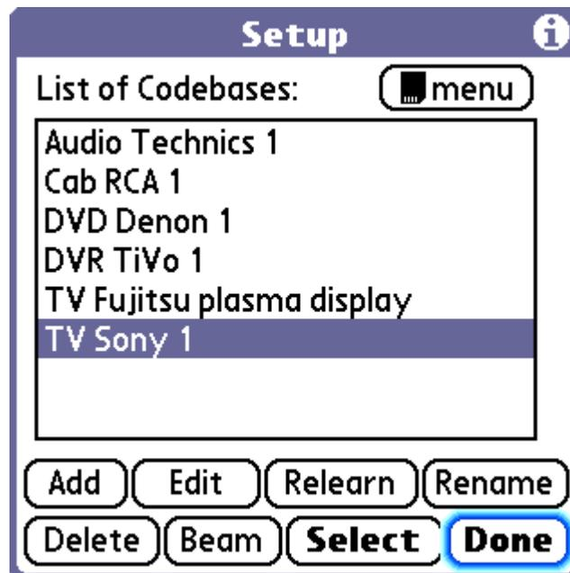
A **codebase** is a database containing the infrared signals that control your equipment. A codebase consists of several **pages** displayed on the screen of your handheld, see the Remote Screen form. Each page consists of the soft **buttons** beaming infrared signals, which control your home devices. **Navigation buttons** allow jumping between pages
