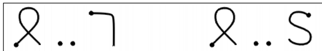
Figure 14-5: Helpful beam debugging shortcuts: toggle beam loopback (left), and serial port IR (right)
