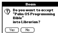
Figure 14-3: This default dialog box prompts the user to accept or reject incoming beamed data.
