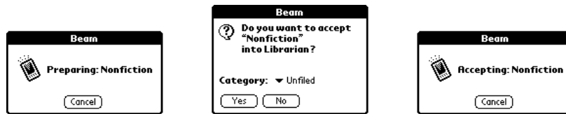
Figure 14-1: Beaming dialog boxes display a description string that describes the data to be transferred. Pictured here are the preparation dialog box (left), a dialog box to prompt the user to accept the data (middle), and the accepting dialog box (right), all of which display the description “Nonfiction.”
