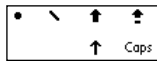
Figure 2-17: The four Graffiti shift states, pictured from left to right, are punctuation, symbol, uppercase shift, and uppercase lock.
