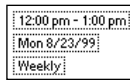
Figure 2-11: Selector triggers display a value that may be edited by the user's tapping on the control.
