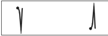
Figure 6-2: The next field (left) and previous field (right) Graffiti strokes allow for rapid data entry on forms containing more than one text field.
