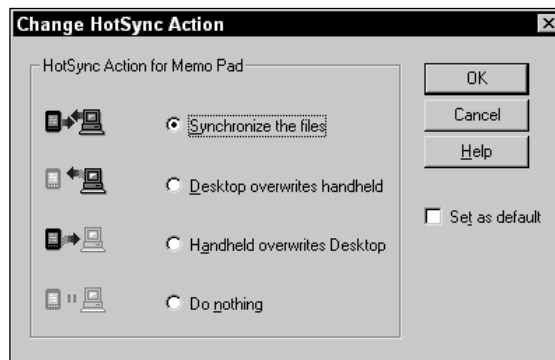
Figure 18-6: The standard Change HotSync Action dialog box, which allows the user to modify a conduit's actions during a HotSync operation
