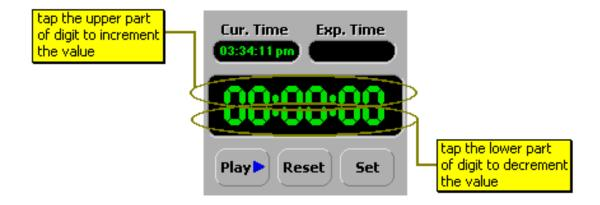
**Method 2:** tap the **aTimer** provided buttons to adjust the timer time.
