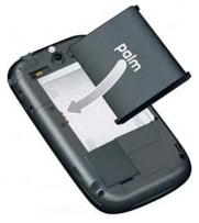
9. To replace the back cover: Insert the **ringer** switch into the hole provided for it on the right side of the back cover.
