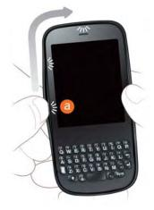
5. Run your thumbnail around the hairline opening to release the bottom-left and bottom clasps. (End at (b).)
