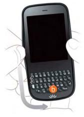
6. Swing the body of the phone out of the back cover as if the right side were a hinge.
