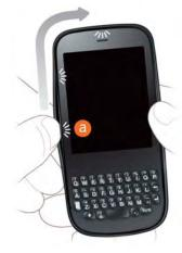
5. Run your thumbnail around the hairline opening to release the bottom-left and bottom clasps. (End at (b).)
