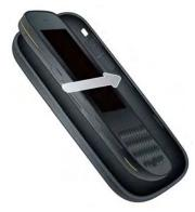
10. Press the back cover and the body of the phone together at each pair of clasps. (You can feel the clasps engage.)
