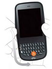
6. Swing the body of the phone out of the back cover as if the right side were a hinge.
