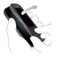
7. Remove the **battery** by sliding your finger under the groove at the side of the battery.
