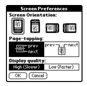
Screen Orientation: Allows you to choose the direction for the eBook text display. Four icons show how you hold the handheld to read the text. The third icon shows landscape mode, which has the handheld's buttons on the right. Landscape orientation is particularly useful for a right-handed person reading with one hand.
